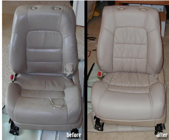
I'm happy to report that the installation of the driver's side leather went much faster than the passenger side. Due to the weight of the motors and stuff, the seat doesn't twist and tip over all of the time.
