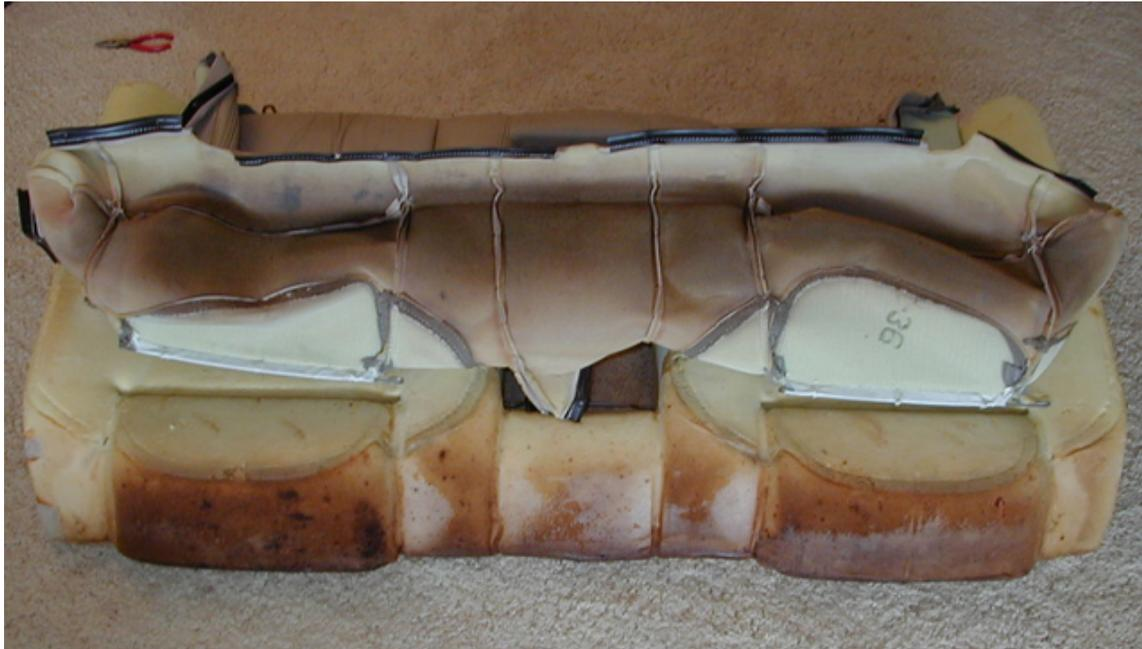
If there was ever a good reason for installing tint with some UV protection, this should be it! This is what the foam looks like underneath the leather in the back seat. You're looking at the top of the seatback, where your head would be if you were sitting in the back seat. The leather here is folded inside out, and you can see the discoloration in both the leather and the foam. The outside of the leather shows no discoloration at all.
